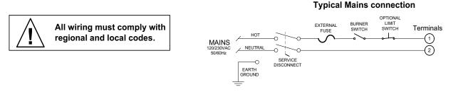
Caution: All safety limit switches must be approved as limit controls and must be wired directly in the circuit of the Flame Safeguard control. The use of electronic switches to close interlock circuits can cause erratic operation.
