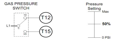
This setup requires that the gas pressure switch be adjusted to  $\frac{1}{2}$  the gas train pressure. The rule of operation is quite simple: The pressure switch will "make" (DI2 high) when gas pressure in the test section exceeds the set pressure; it will "break" (DI1 high) when the gas pressure falls below the set pressure.
