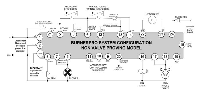
EXAMPLE WIRING DIAGRAM FOR BURNER w/ DIRECT IGNITION
